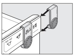
■ From the edge of each drawer, slide the markers onto the guide runners.
